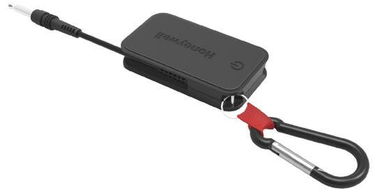
*Supporting DEX and Bluetooth® Low Energy standards, the Honeywell DEX Wireless Adapter is an affordable, maintenance-free DEX solution – no charging required.*
